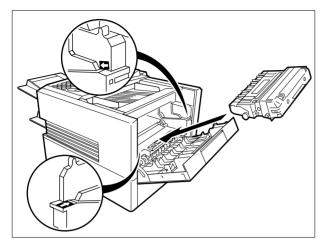
Align the arrow and the projection on both sides as shown and insert the Toner Cartridge into the machine.
